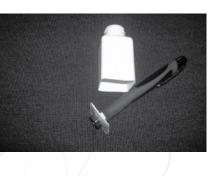
(Left) What you're looking at is a pill bottle with the bottom cut out. The bottom was trimmed to fit inside the bottle and inserted between two nuts and threaded onto a bolt. The barrel of this ink pen, it served the purpose of a plunger.
