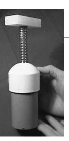
Another design of a homemade soil blocker, with a completed soil block. (Plans on how to make it >)
